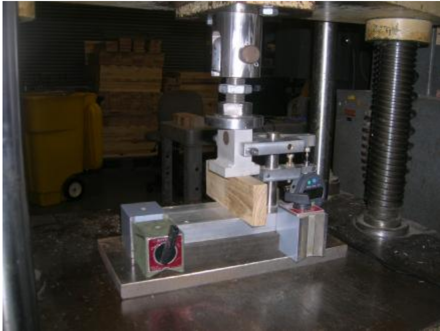
Figure 2. Compression perpendicular-to-grain test being conducted
