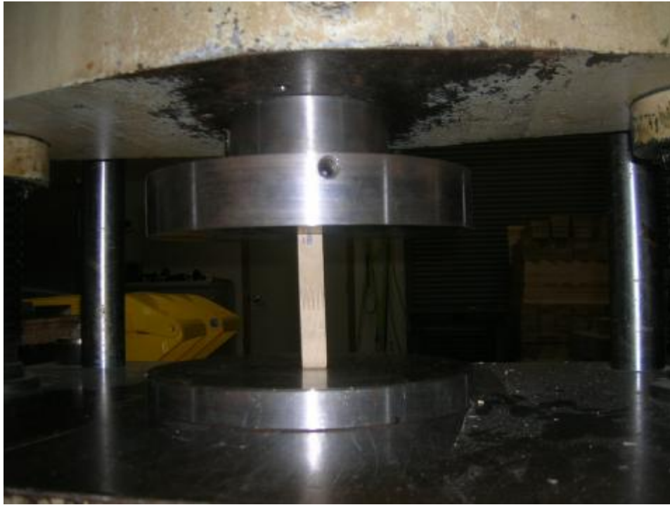
Figure 1. Compression parallel-to-grain test being conducted
