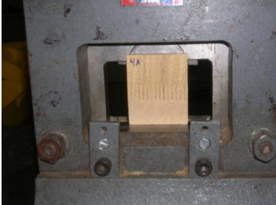
Figure 3. Shear parallel-to-grain test being conducted
